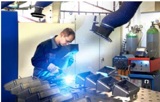
Welding departments with direct air extraction.
